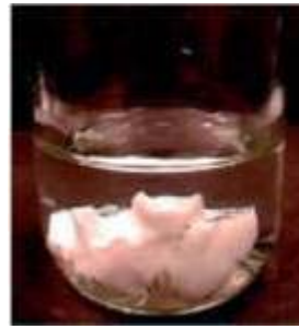
Krytox® grease in hydrocarbon solvent is not dissolved.
