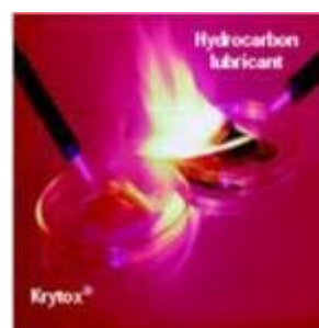
Hydrocarbon-based lubricants burn; Krytox® does not.
