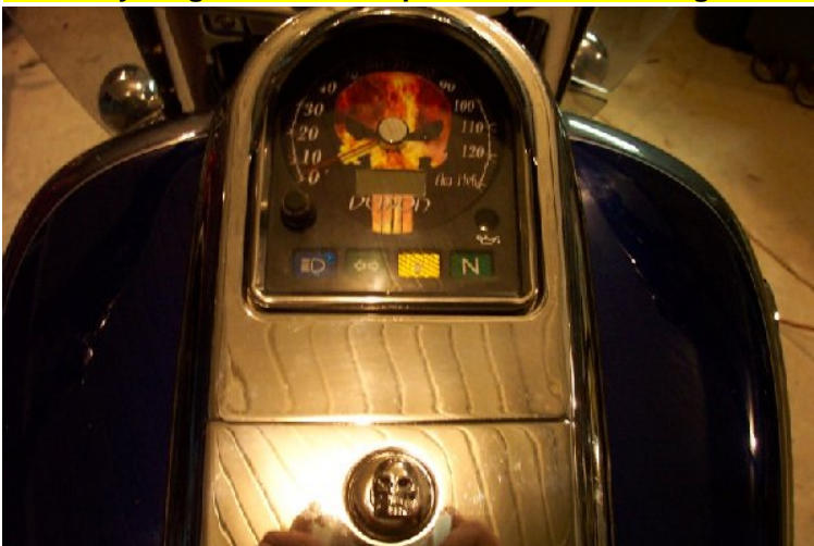
Install new speedo face, screws and needle stop. Put everything on in reverse procedure from taking off.
