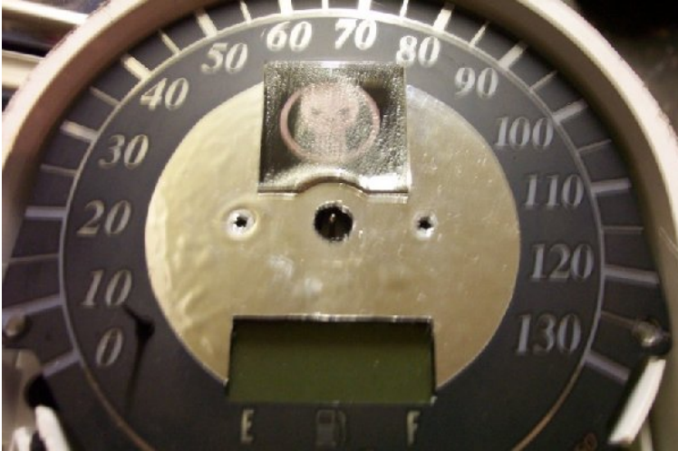
Remove the speedo face and the needle stop pin at this point so you can reuse it on your new dial.
