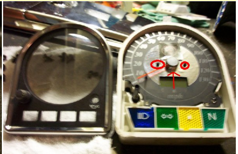
Bottom housing has 2 screws that need removed and speedo needle needs removed. CAUTION: needle is fragile and will break if you're not careful. A chip puller works the best to remove the needle but a fork works well.
