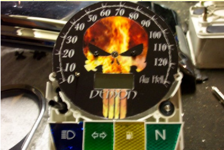
Install new speedo face, screws and needle stop. Put everything on in reverse procedure from taking off.
